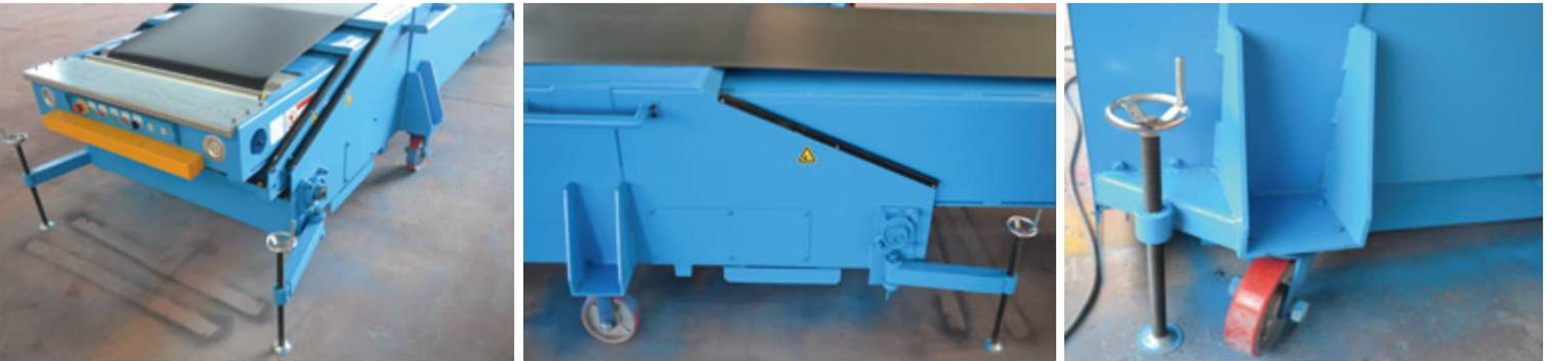
Bolts and feet fix the conveyor Blue paint RAL 5015 Casters and feet are installed
